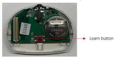
2. Hold down the button, after red light flash 3 times, means reset successfully, as below
