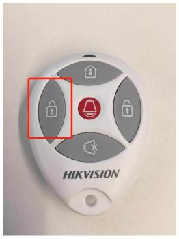
2) Hold down the button, after **Red** light flash 3 times, means reset successfully, as below.
