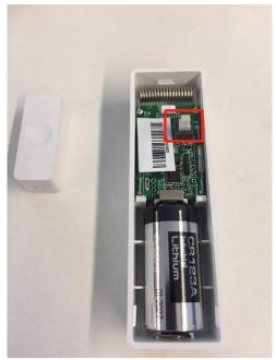
2) Hold down the button, after **Red** light flash 3 times, means reset successfully, as below.
