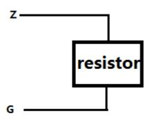
If "Zone Fault" disappears, we can confirm it is a wiring fault between detector and control panel. Check wire poor contact, short circuit, open circuit between detector and control, or signal cable is too close to power cable. After all these wiring issue have checked, but control panel is still in "zone fault" status, go on next step.
