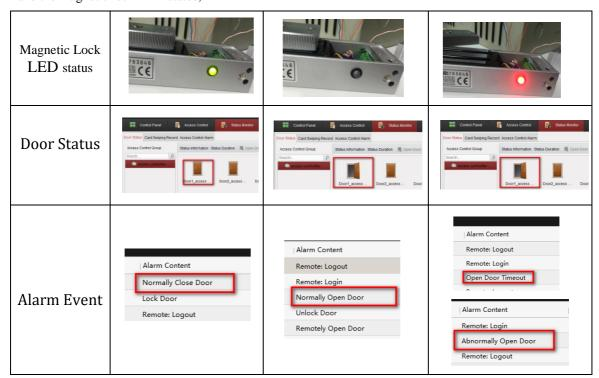
**NOTE:** Abnomal in *Magnetic lock LED status* part could be displaied in following scenario, open door timeout, abnomally open door(by force), as well as not standard installation cuasing armature plate and lock body contact are not fully fitted.
