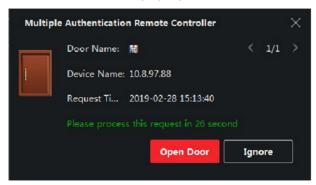
Figure 7-6 Remotely Open Door
