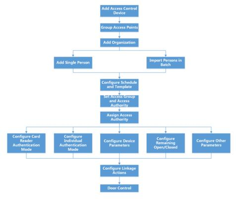
Figure 7-1 Flow Chart of Access Control
