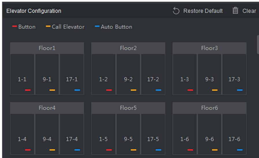
Figure 7-7 Relationship between Relay and Floor
