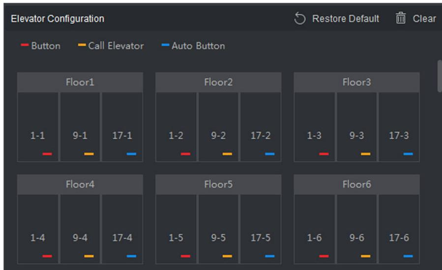
**Figure 15-11 Relationship between Relay and Floor**
