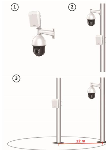
Figure 9-17 Scenario of One-Point Calibration
