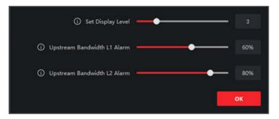
**Figure 18-2 Set Topology Parameters**
