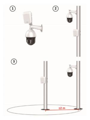
Figure 9-18 Scenario of One-Point Calibration
