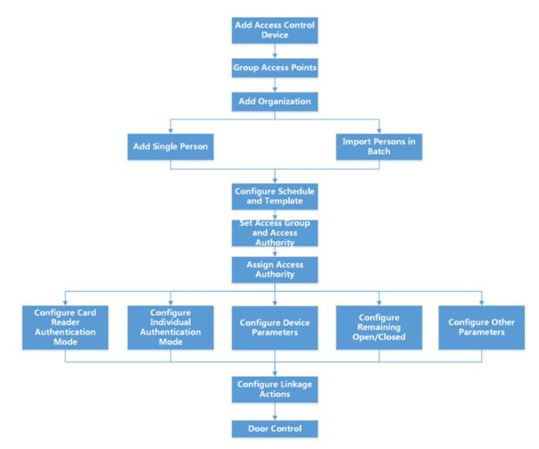
Figure 16-1 Flow Chart of Access Control
