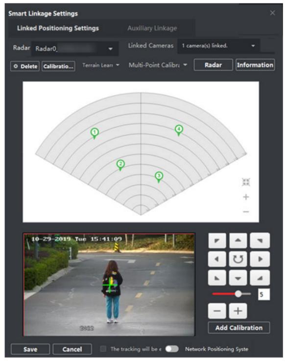
Figure 10-23 Multi-Point Calibration Radar Page
