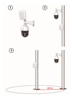
Figure 10-18 Scenario of One-Point Calibration
