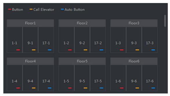
Figure 16-10 Relationship Between Relay and Floor
