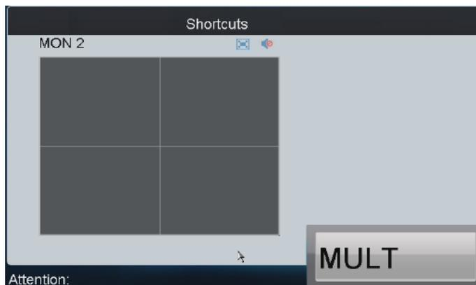
3. Press the **Num + CAM** keys to select the input camera.
