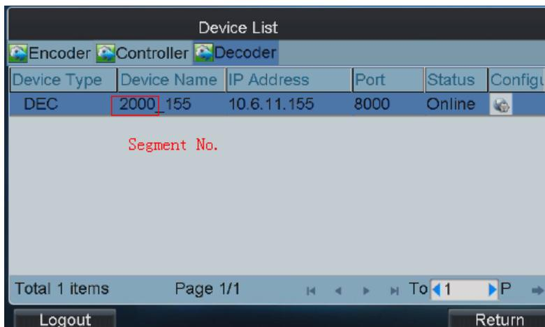
2. The decoder should cooperate with IVMS-4200 Video Wall Client Software when its firmware version is V3.5.0. For example, you can open two window in video wall, if you want to display the video on **Screen 2**, Press **2002 + MON** keys to select Screen 2 of the video wall.
