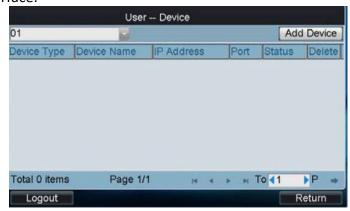
Step12. Click **Add Device** to enter the "User-Add Device" interface. Select the device by clicking the checkbox, and click **Add** to add the device for the current user. And the added device (s) for the current user can be displayed on the "User List" interface.
