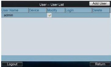
Step10. In the User List interface, click **Add User** to enter the "Add User" interface. Input the user name, password and verify the password. Finally, click **Add** to finish the adding of user.
