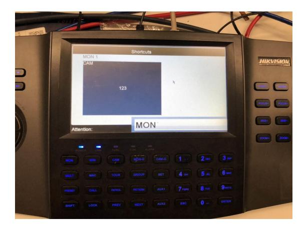
Step 7: press number + CAM button, you can change other camera to this window to display.
