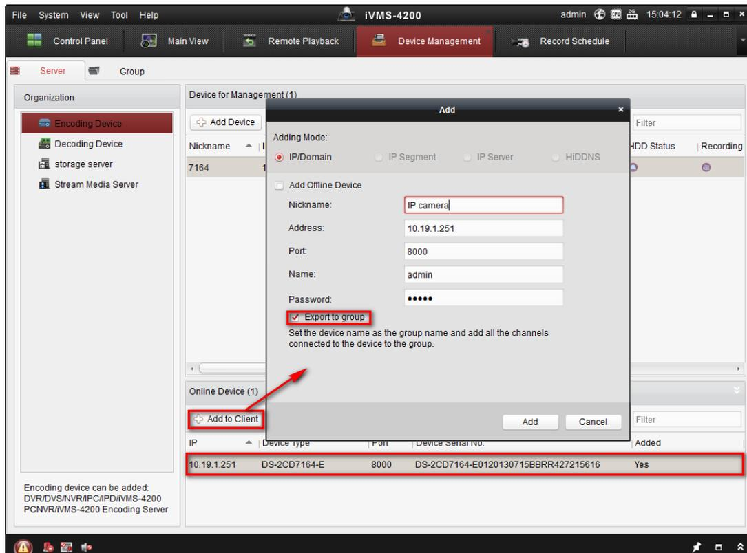
3, Select the device and click **Remote Configuration-> Configuration-> General->** fill in the Multicast Address.
