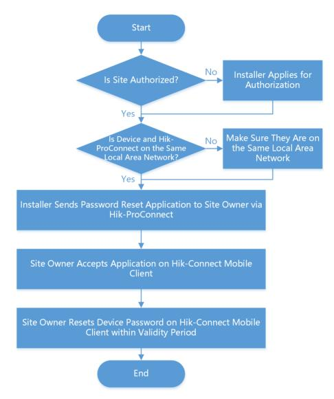
Figure 7-12 Flow Chart of Resetting Device Password
