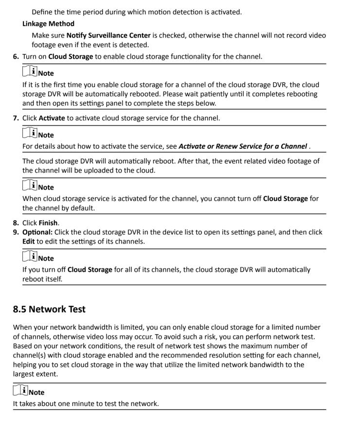
You can click the cloud storage device in the device list to open the device settings panel, and then click  $\bigcirc$  **Start** to start network test.
