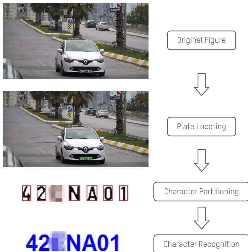
Figure 1 Plate Recognition Flow
