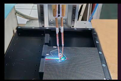
Repairing LED lamps has always posed challenges for HOB products due to the glue layer on the lamp board surface. Now, Hikvision introduces an HOB LED lamp repair machine to address this issue.
