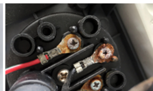
Malfunction due to corrosion
