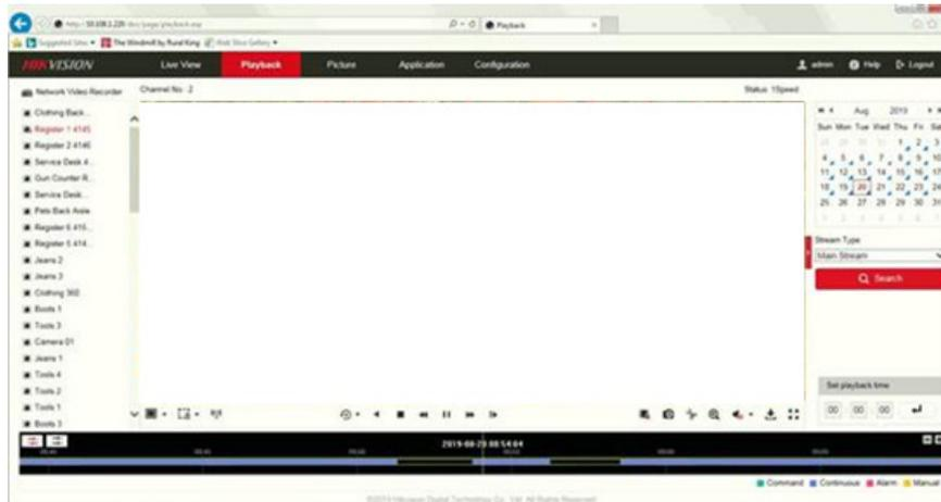
Figure 2, Time Bar Should Be Continuous Blue, but Shows Blank Gap
