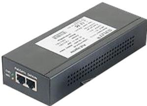
Single port POE midspan, Injection Voltage 56 Vdc , Max. 60W, Input 110/240 VAC, 50/60Hz, 2A Max
