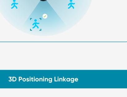
Draw a box on **Static lens view**, then **PTZ lens** will automatically zoom in to that area.
