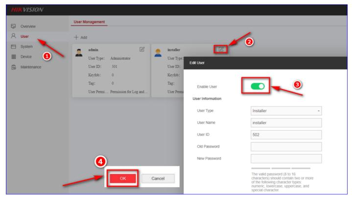
Step 3: Log out the webpage, then log in again using installer account, please be noted, the default password of the installer account is installer12345 and it will ask you to change the default password automatically.
