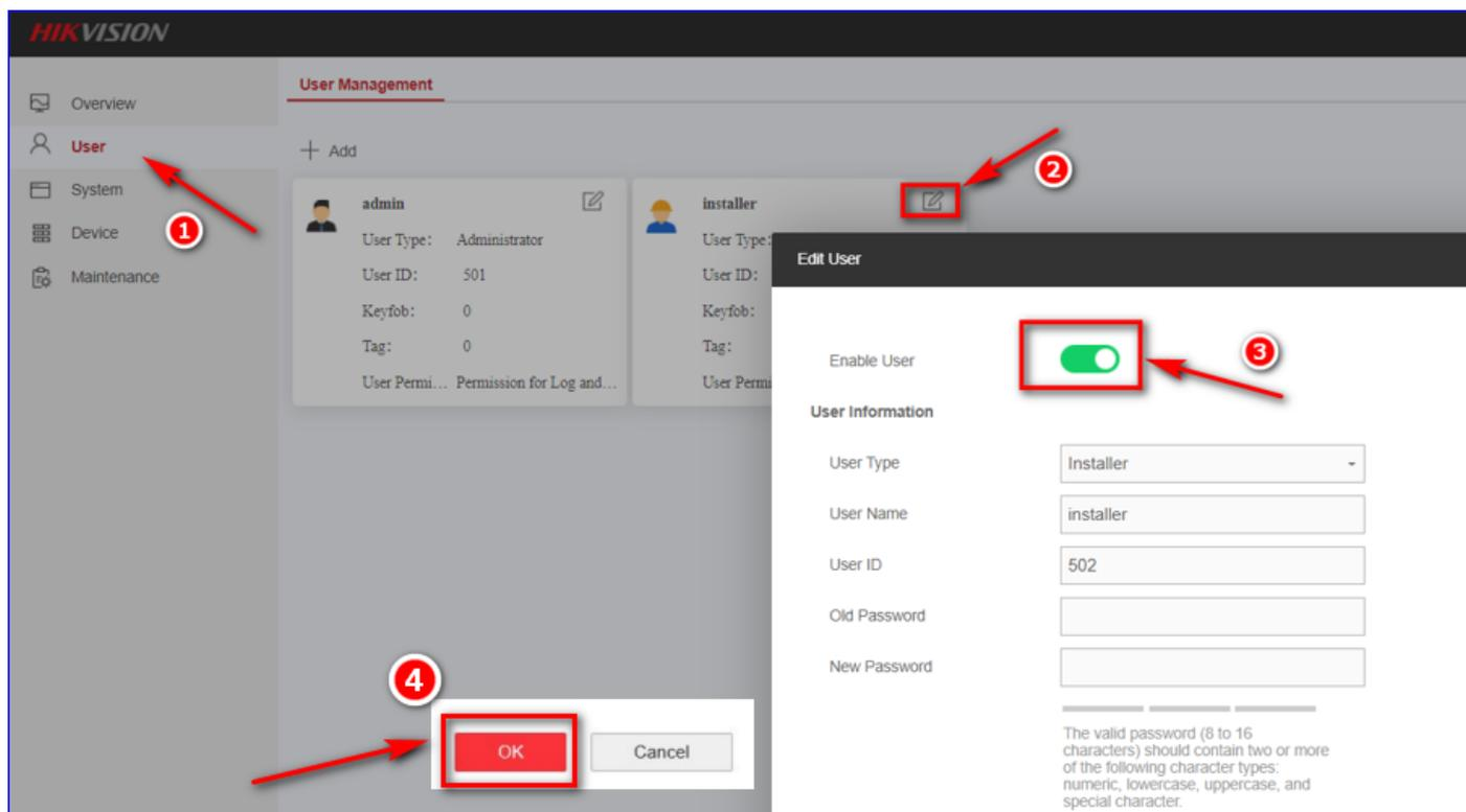
Step 3: Log out the webpage, then log in again using installer account, please be noted, the default password of the installer account is installer12345 and it will ask you to change the default password automatically.
