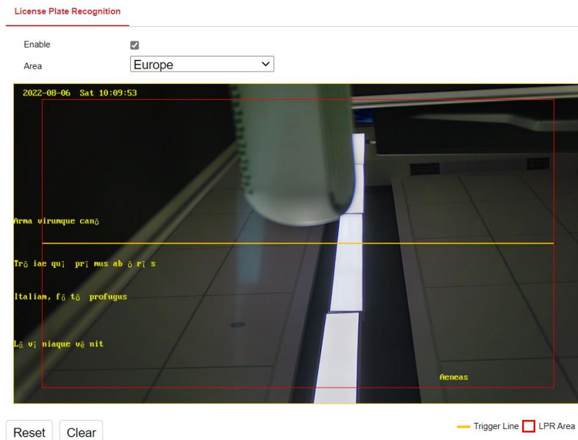
Figure 9-2 License Recognition Area and Trigger Line
