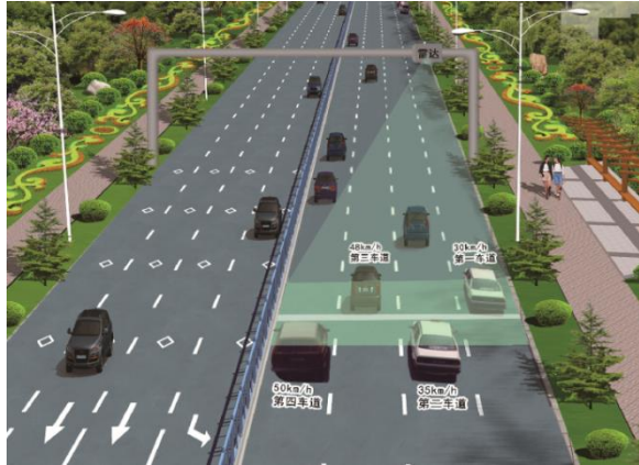
Figure 2.5: The radar installation is deviated from the above center of the lane but in the lane.
