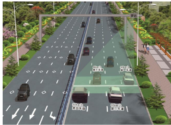
Figure 2.6: The radar is installed above and outside the lane.
