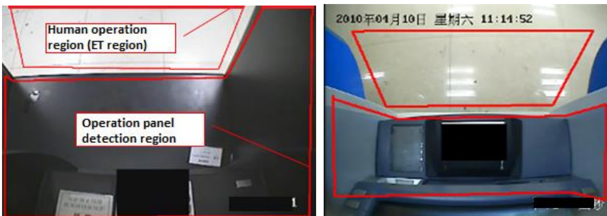
Figure 1-1 Camera Installation for Panel Mode
