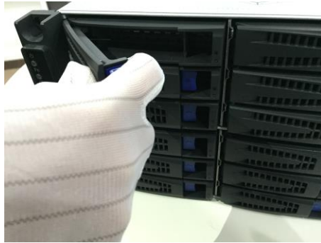
Figure 3-1 Pull Out Dummy HDD
