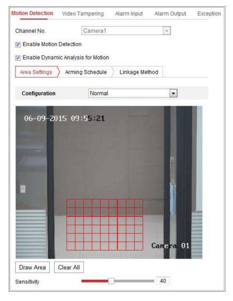
Figure 10-1 Enable Motion Detection
