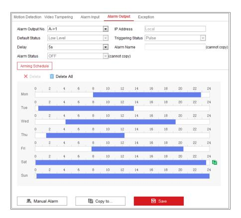
Figure 10-8 Alarm Output Settings
