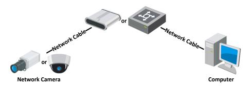
Figure 2-2 Connecting via a Switch or a Router
