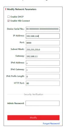
Figure 2-5 Modify the IP Address
