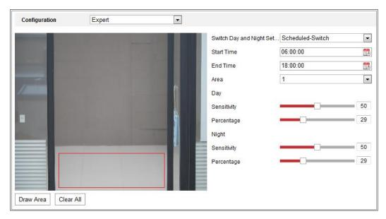
Figure 10-5 Expert Mode of Motion Detection
