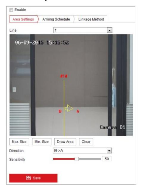
Figure 10-19 Line Crossing Detection
