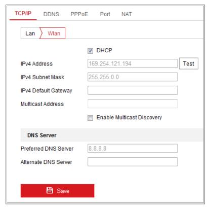
Figure 4-11 Setting WLAN Parameters
