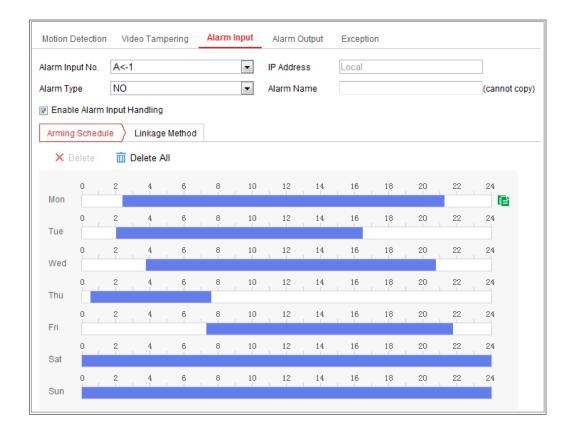
Figure 10-7 Alarm Input Settings
