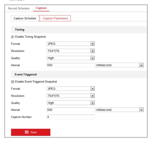
Figure 11-5 Set Capture Parameters
