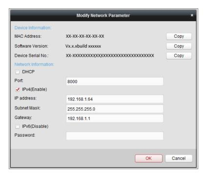
Figure 2-9 Modifying the Network Parameters
