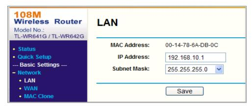
Figure A.2.2 Set the LAN parameters
