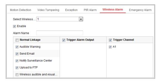
Figure 10-9 Setting Wireless Alarm
