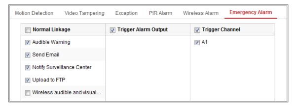
Figure 10-13 Setting Emergency Alarm
