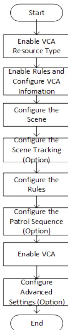
Figure 6-1 Flow Chart of Perimeter Protection Configuration
