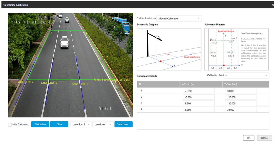
**Figure 3-2 Manual Calibration**
