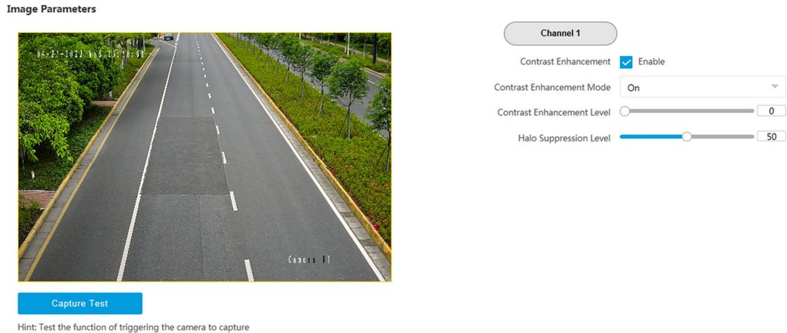
**Figure 2-3 Set Captured Image Parameters**
