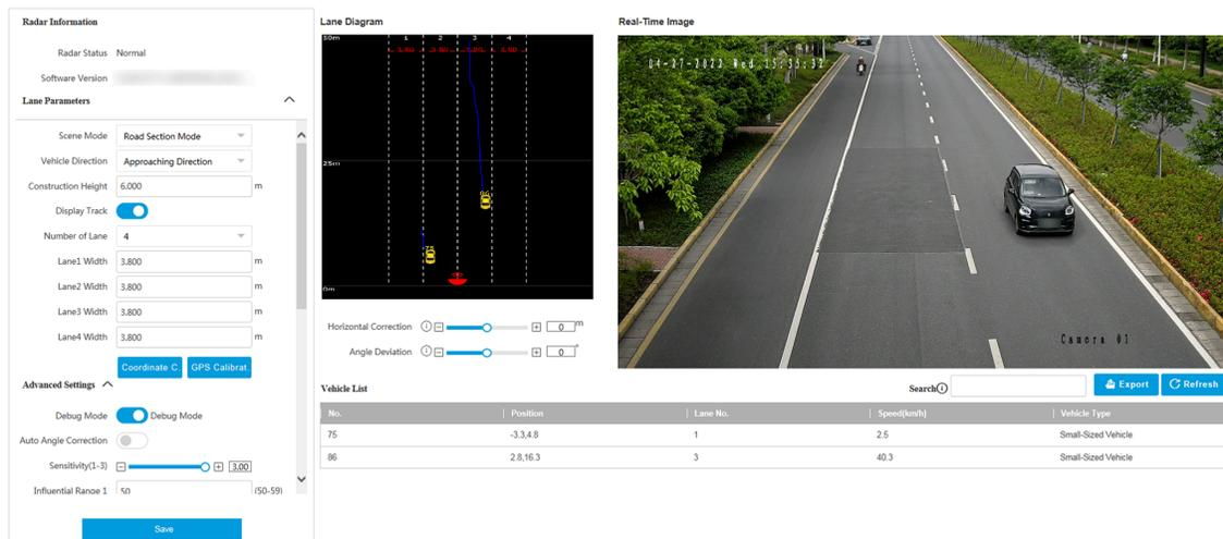
Figure 3-1 Set Radar Parameters
