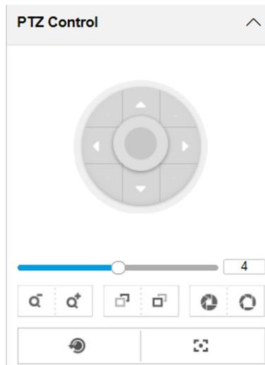
**Figure 5-1 PTZ Control Panel**
