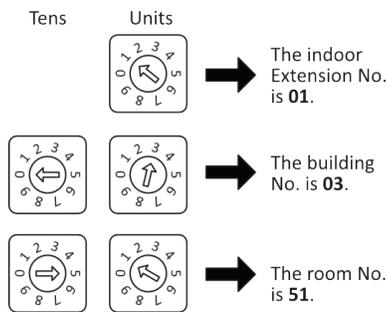
**Figure 4-4 Example: DIP Switch of Indoor Station**
