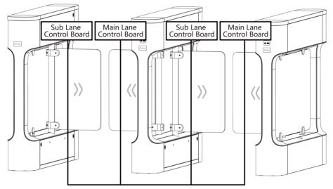
Figure 4-4 Connect Interconnecting Cable
