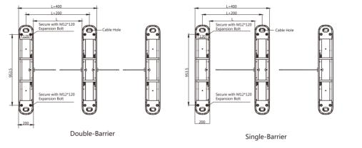
Figure 3-6 Installation Footprint
