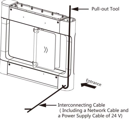
Figure 4-8 Pull out Interconnecting Cable
