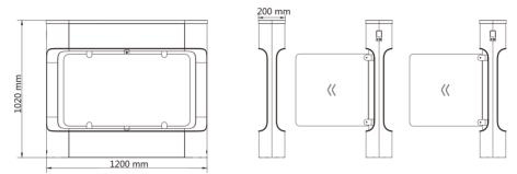
Figure 3-5 Single-Barrier Dimension
