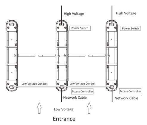
Figure 2-2 System Wiring Diagram (General Wiring)
