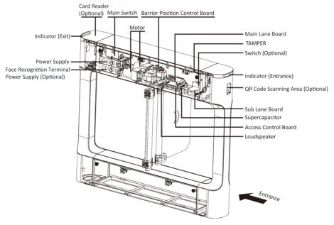
Figure 4-1 Components Diagram 1
