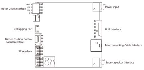
Figure 4-12 Sub Control Board Terminal
