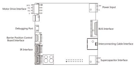
Figure 4-11 Main Control Board Terminal
