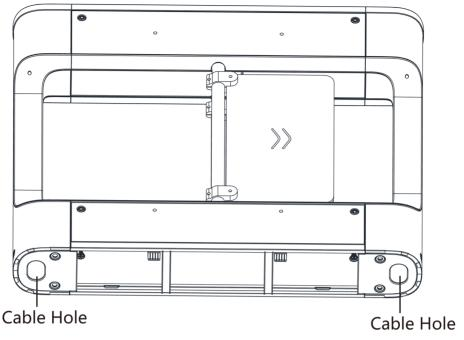
Figure 4-3 Cable Hole of Interconnecting Cable
