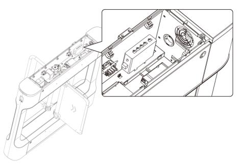
Figure 4-10 Network Switch Position
