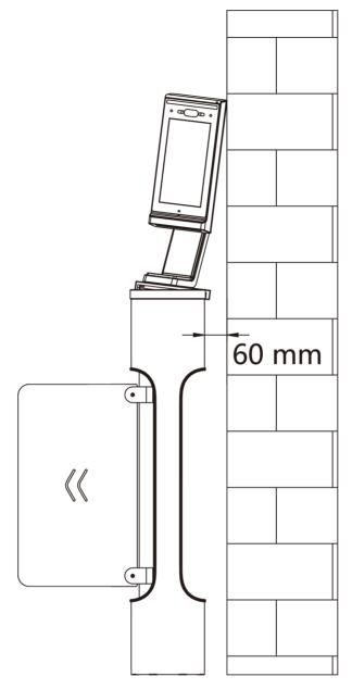
Figure 3-3 Installation Distance (With Face Recognition Terminal)
