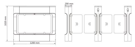
Figure 3-4 Double-Barrier Dimension
