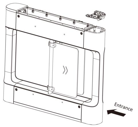
Figure 4-7 Dissemble Card Reader Module
