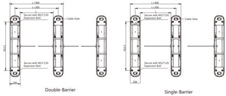
Figure 2-1 Hole Position Diagram
