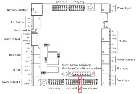
Figure 5-1 Initialization Jumper Cap
