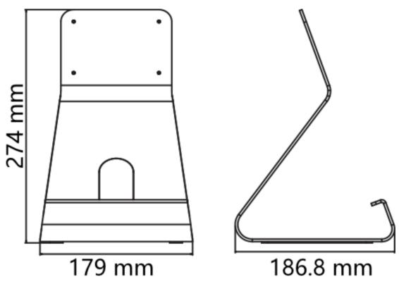
Figure 3-14 Base Mounting Bracket
