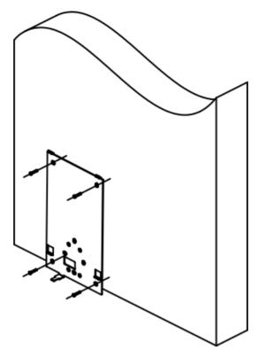
Figure 3-10 Install Mounting Plate
