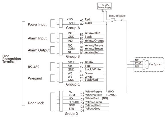
Figure 4-6 Wiring Device
