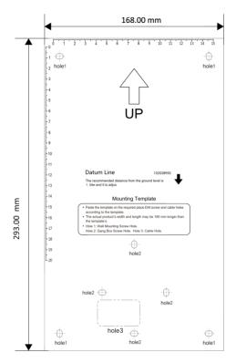
**Figure 3-9 Mounting Template**
