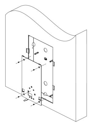
Figure 3-6 Install Mounting Plate
