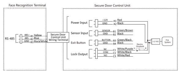
Figure 4-5 Wire Secure Door Control Unit
