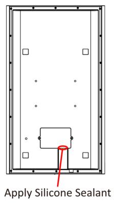
Figure 3-3 Apply Silicone Sealant
