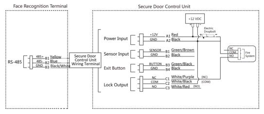
Figure 4-7 Wiring Secure Door Control Unit
