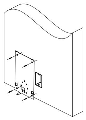
Figure 3-2 Install Mounting Plate
