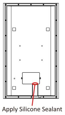
Figure 3-11 Apply Silicone Sealant
