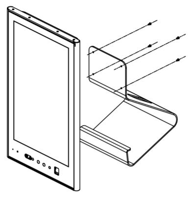
Figure 3-15 Remove Back Cover Plate
