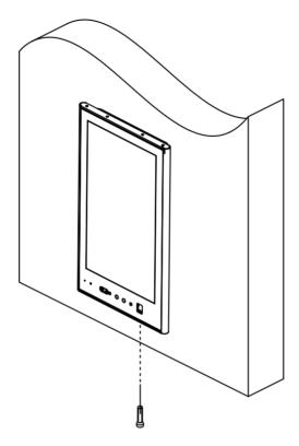
Figure 3-4 Secure Device
