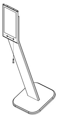
Figure 3-17 Install Device
