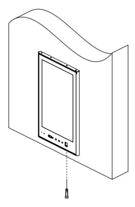
Figure 3-13 Secure Device
