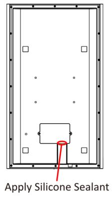
Figure 3-7 Apply Silicone Sealant
