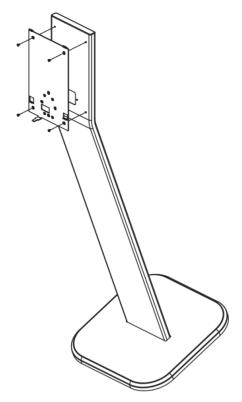
Figure 3-16 Install Mounting Template
