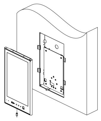
Figure 3-8 Secure Device
