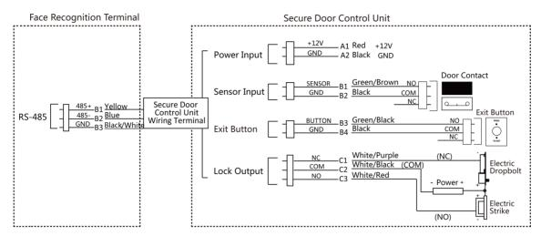
Figure 4-3 Secure Door Control Unit Wiring
