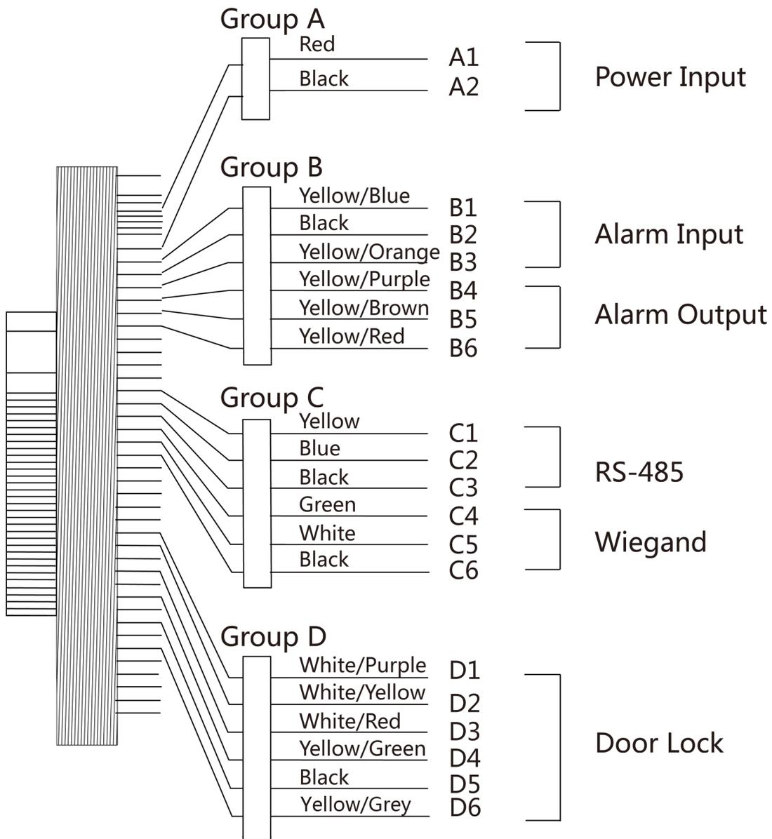
Figure 4-1 Terminal Diagram
