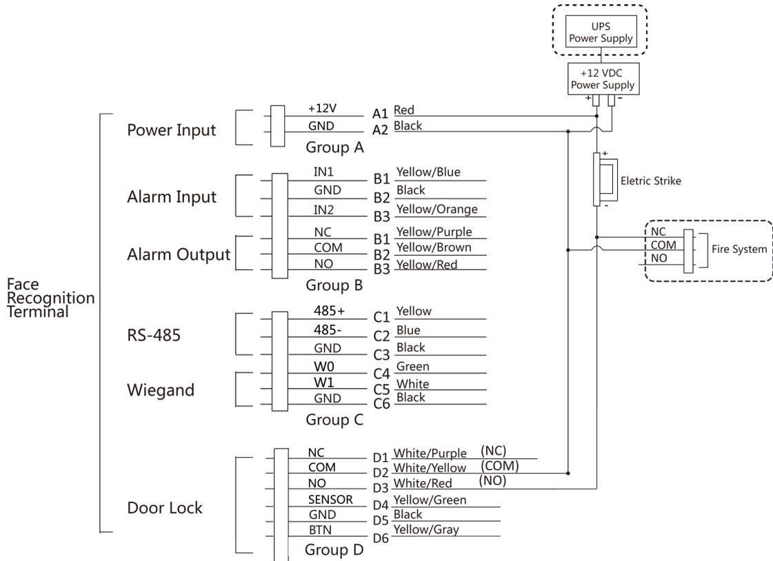
**Figure 4-8 Device Wiring**
