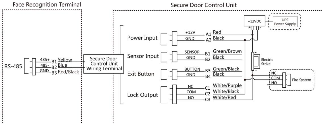
**Figure 4-9 Wiring Diagram**
