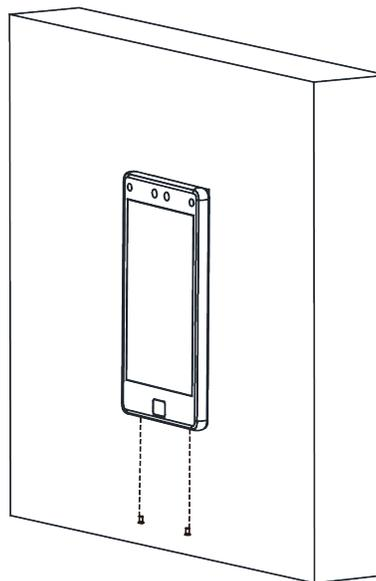
**Figure 3-4 Secure Device**
