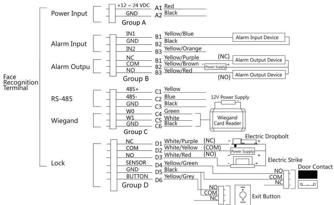
**Figure 4-2 Device Wiring**
