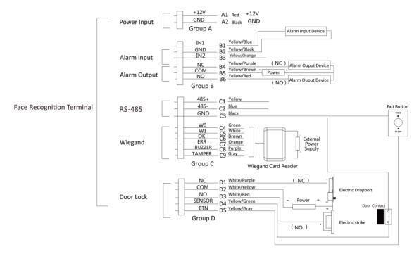
Figure 4-2 Device Wiring
