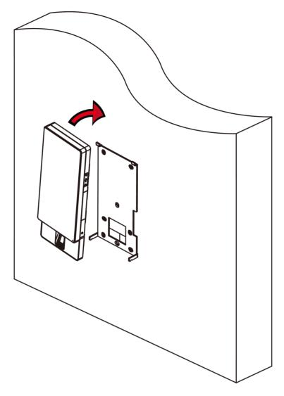
Figure 3-12 Install Device
