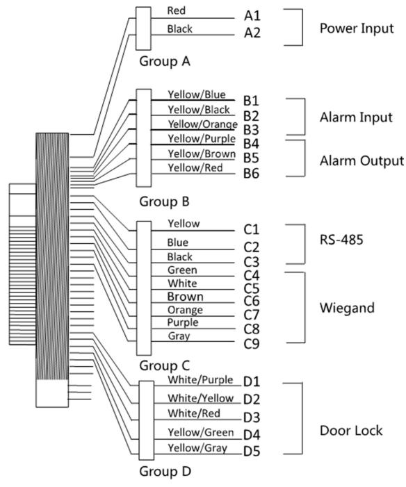
Figure 4-1 Terminal Diagram
