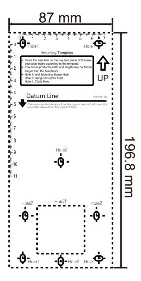
**Figure 3-7 Mounting Template**
