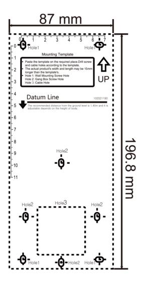
**Figure 3-1 Mounting Template**
