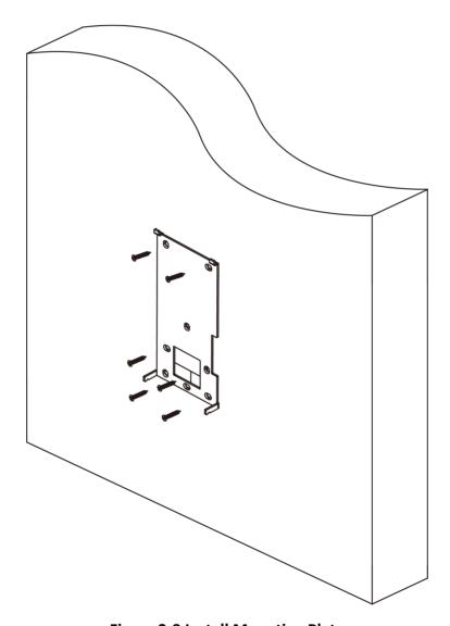
Figure 3-9 Install Mounting Plate
