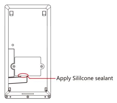
Figure 3-3 Apply Silicone Sealant
