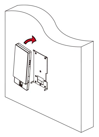
Figure 3-5 Install Device
