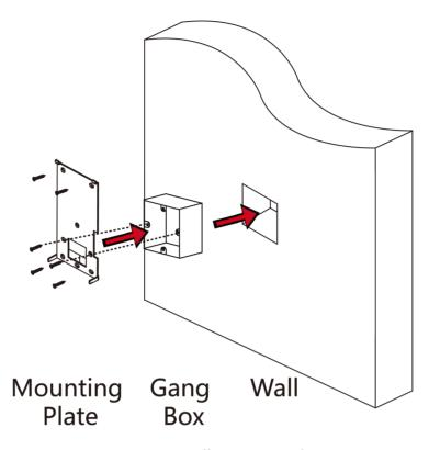
Figure 3-2 Install Mounting Plate
