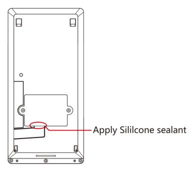
Figure 3-10 Apply Silicone Sealant
