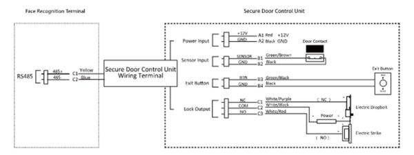
**Figure 4-3 Secure Door Control Unit Wiring**
