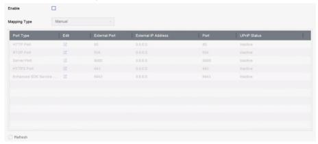
Figure 11-2 Port Mapping Setting
