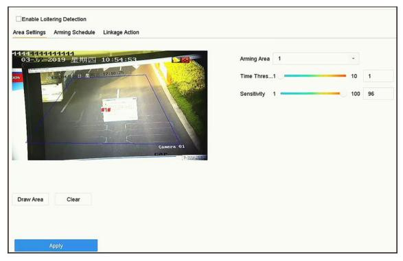
**Figure 6-9 Loitering Detection**
