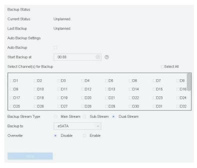
Figure 11-6 Configure eSATA for Auto Backup
