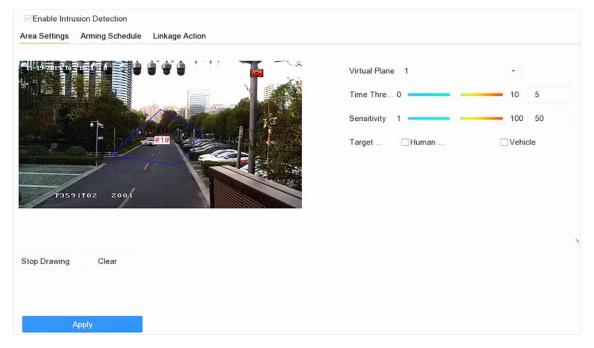
**Figure 6-6 Intrusion Detection**
