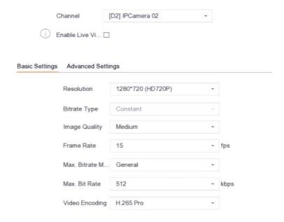
**Figure 3-6 Transcoded Live View**
