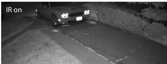
IR on In the absence of a vehicle or person, the camera uses only IR light.
