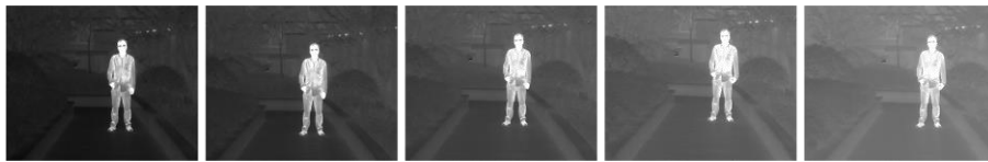
Figure 3-4 Adjust Brightness in White Hot Mode
