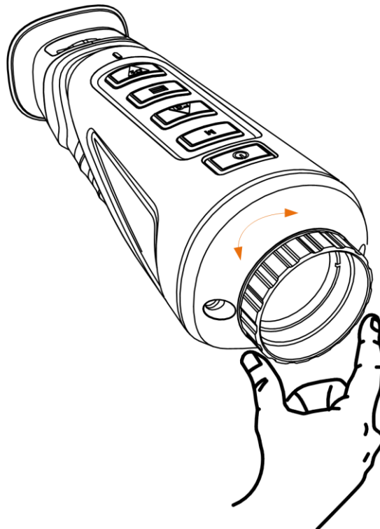
Figure 3-3 Adjust Objective Lens
