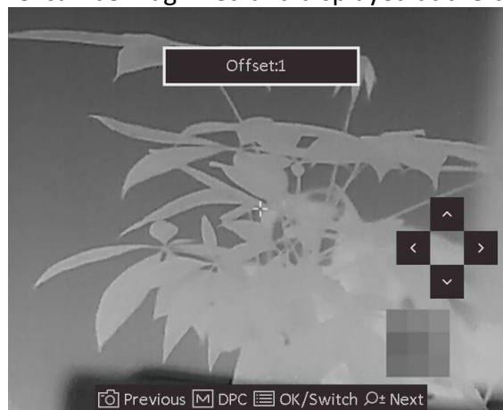
Figure 3-5 Correct Defective Pixel
