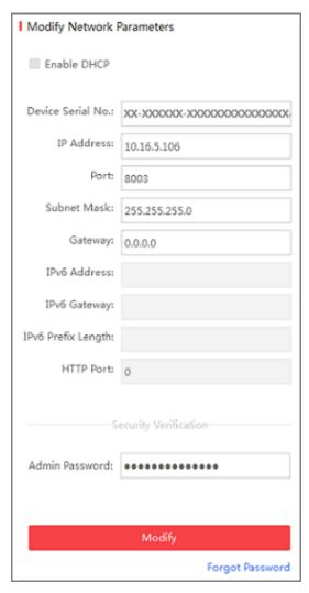
Figure A.1.2 Modify Network Parameters
