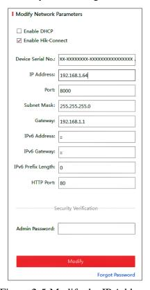
Figure 2-5 Modify the IP Address
