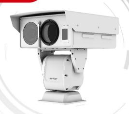
Hikvision DS-2TD8167-190ZE2FL/W Thermal & Optical Bi-spectrum Network Stable PTZ equipped with built-in GPU which supports intelligent perimeter protection algorithm, can realize high-precision VCA detection and real-time alarm. It is applied to frontier protection scenes, such as airport, railway, farm, and parking lot. The pre-alarm system helps you discover unexpected events immediately and protects your property.
