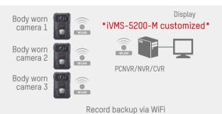
Docking stations charge Body Worn Cameras and download captured video data when docked via USB port. An external LCD screen provides a dashboard for device management, maintenance and secured data storage.
