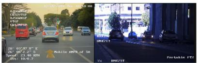
ANPR & GPS position & battery capacity overlay appear
