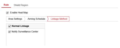
8. Configure **Shield Region** if necessary. Shield Region is used to shield the area which doesn't want to count the heat map statistics. Up to 4 shield regions are configurable.
