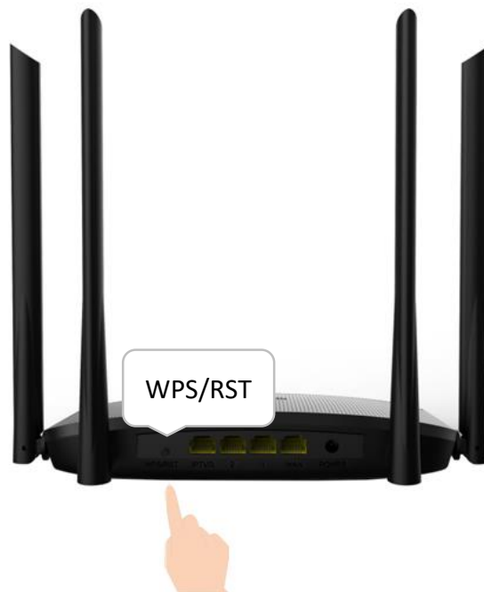
Figure 7-14 Reset the router using the reset button
