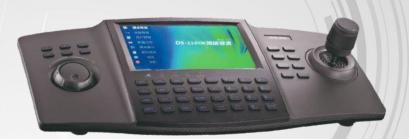
DS-1100KI Network Keyboard can be used to control the camera/speed dome, display of decoded video on TV wall, control of matrix, as well as support 1 channel of video view at up to 1080P resolution. Designed with touch screen, it is easy to operate and configure settings.
