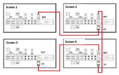
Connect the infrared probe to IR IN of Screen 1(the source of control signals), and put the other side on the front of LCD display unit, making sure the infrared signals from remote control can be detected
