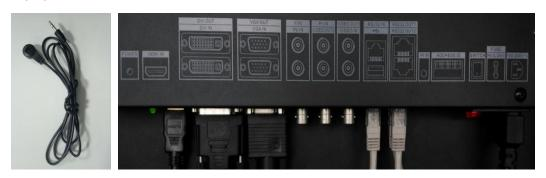
Control cables are for loop output and splicing display, it transmit control signals between screens, standard cables are network cable with RJ45 interfaces, connect the RS232 OUT1 of x with the RS232 IN of x+1, as the picture below shows
