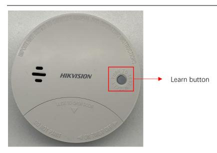
2. Hold down the button, after red light flash 3 times, means reset successfully, as below
