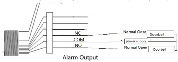
2. Set alarm output linkage in Access Control module, add linkage for doorbell ring event and set alarm output as Close or Open (depends on doorbell type), and click "Save".
