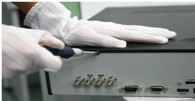
Figura 2.1 Remova a tampa
