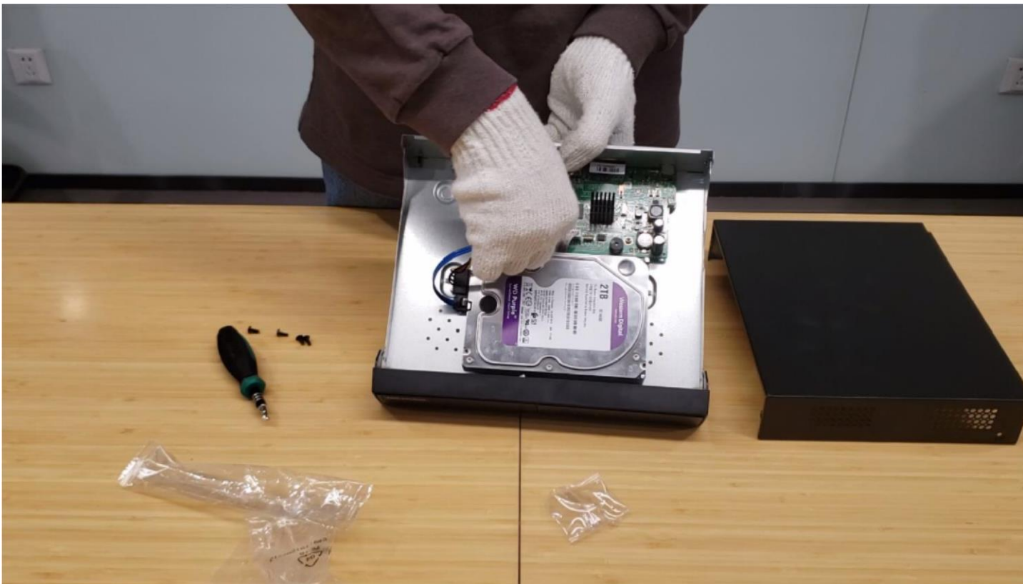
e) Install the cover back
