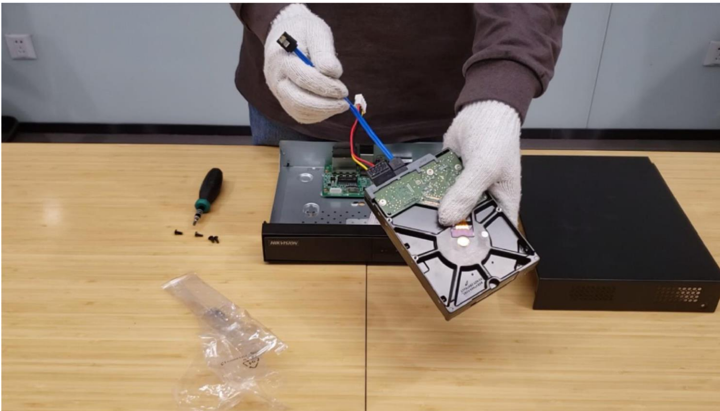
c) Fix HDD to NVR bottom
