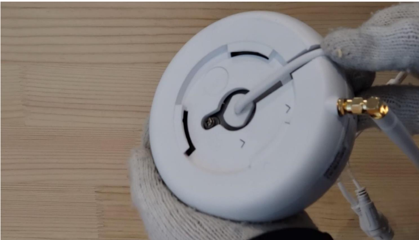
g) Fix camera to the adaptor
