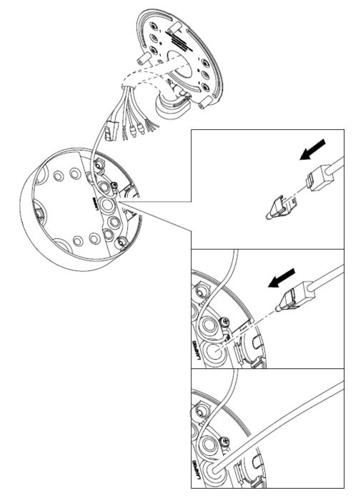
3) When the cable passes through the silicone waterproof cap of the junction box, it shall be guaranteed that single line with single port, do not multiple lines shared with the same outlet port
