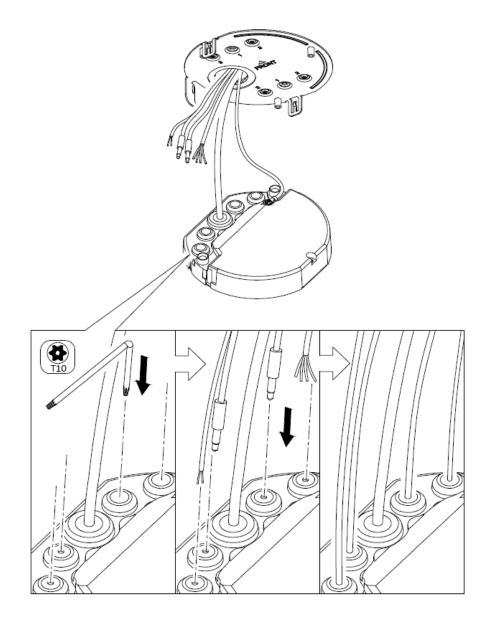
3) When the cable passes through the silicone waterproof cap of the junction box, it shall be guaranteed that single line with single port, do not multiple lines shared with the same outlet port.
