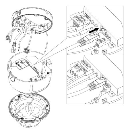
5) When installing the junction box and shell, pay attention to tight press the sealing ring.
