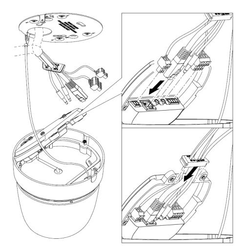
4) When installing the junction box and shell, pay attention to tight press the sealing ring.
