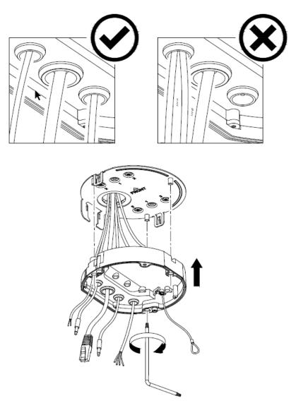
Wiring steps as shown below (Cable waterproof wiring diagram refer to 26xx series).
