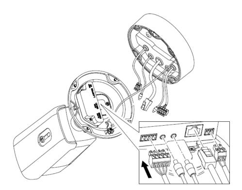
5) Cable waterproof wiring diagram :
